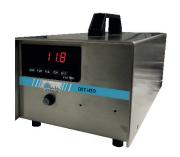
Trace moisture monitoring in gaseous samples
