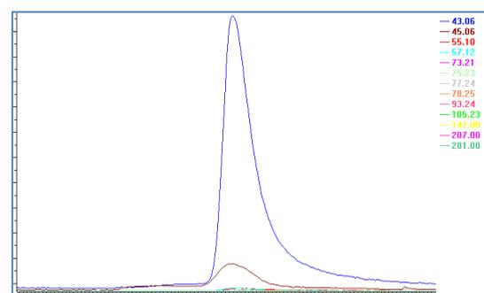
Fig. 3: Graphic obtained with the mass spectrometer. The different ions are displayed versus the time of analysis
