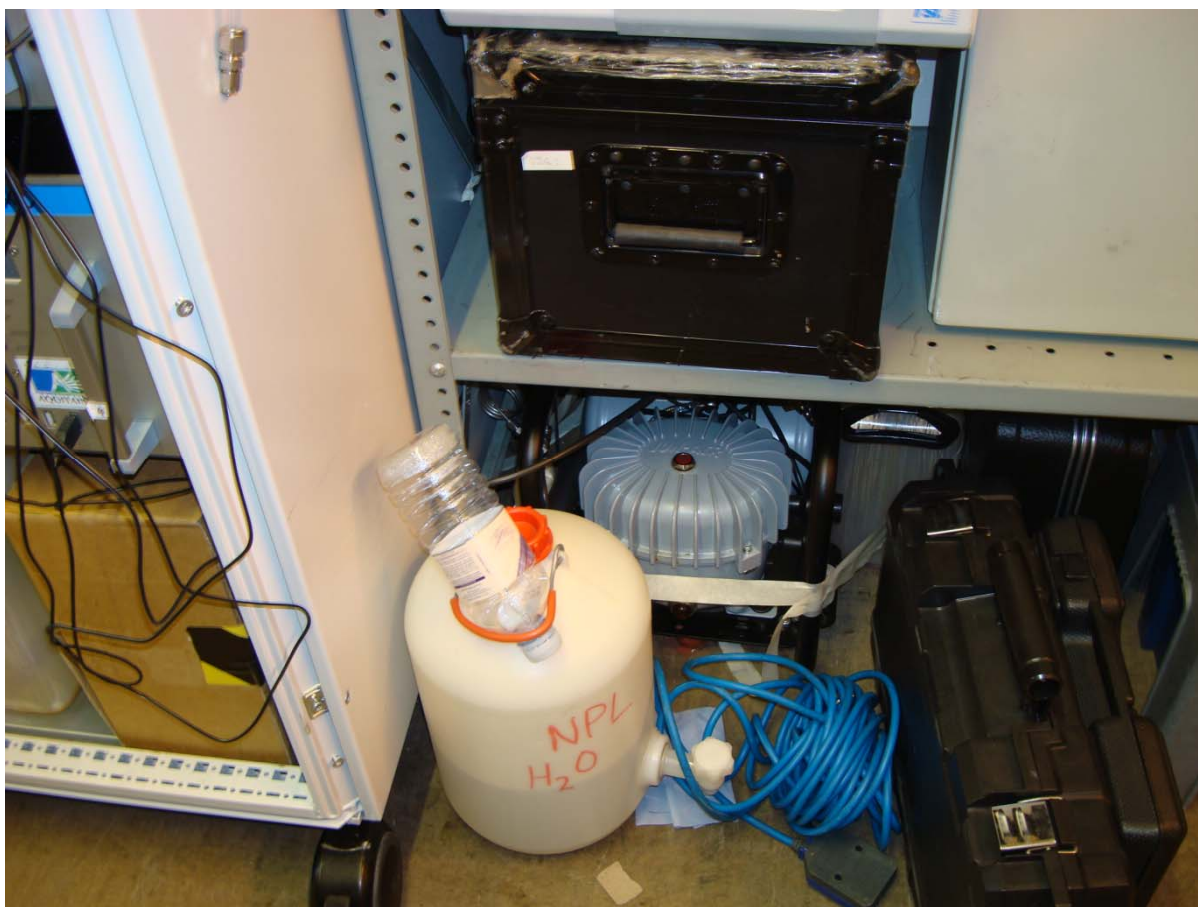
Figure 22: Photograph showing the air generator employed by the CAMs measuring VOCs with a flame ionisation detector.
