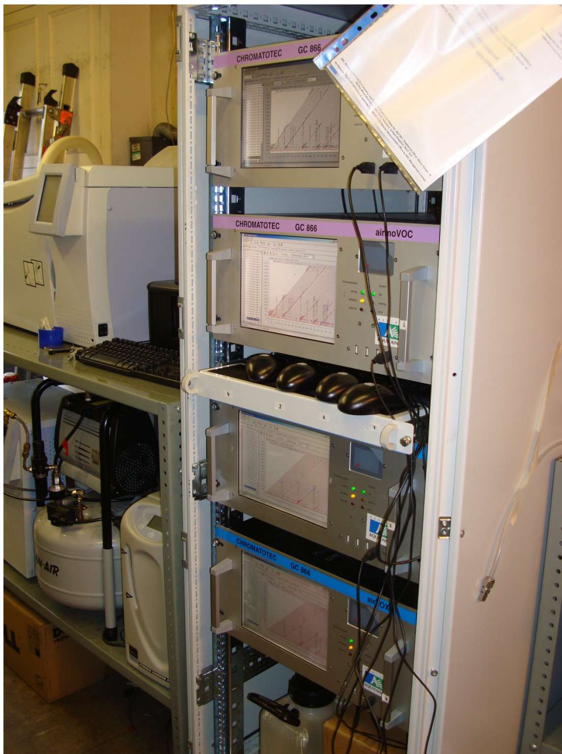
Figure 20: Photograph showing the four CAMs sampling in the field test
