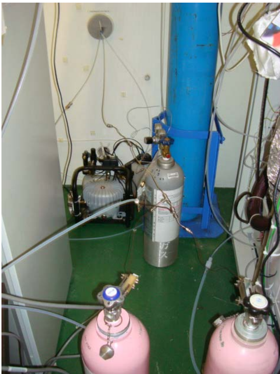
Figure 18: Photograph showing the zero air generator (Compressor, airmoPURE 45 psi) located outside NPL's environmental chamber, together with determinand gas mixtures being piped to the test manifold.
