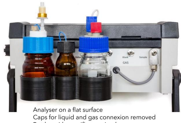
Caps for liquid and gas connexion removed Bottles with specific caps in place Gas at atmospheric pressure Then turn on the analyser
