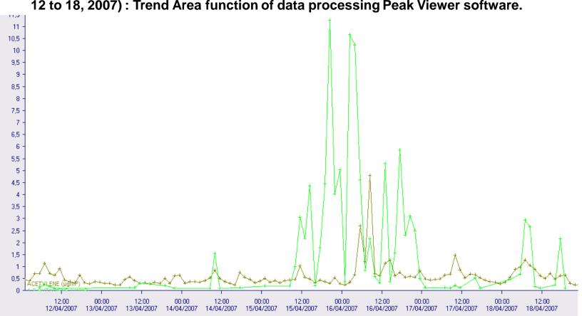
airmoVOC C2-C6 : Follow-up of acetylene concentration (in  $\mu$ g/m3) over one week (April 12 to 18, 2007) : Trend Area function of data processing Peak Viewer software.
