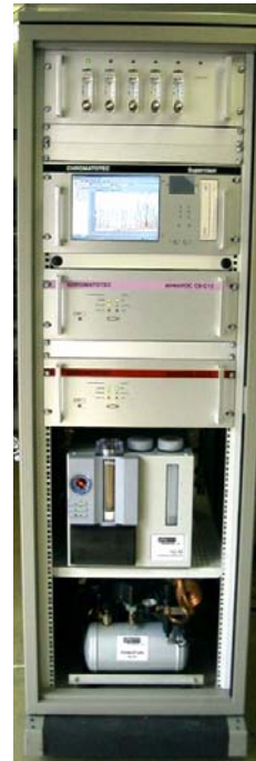
AirmOzone System with its supervisor in 5 U rack and its multiplexer
