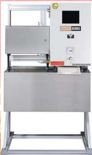
Thanks to an internal or external PC (required for safety areas), it is possible to collect data with the software Windows XP. That allows transferring Concentrations, TOS calculations and status (calibrations, streams, default analyser) by the Modbus protocol to the control room
