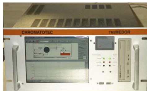
New analyzer for detection of volatile Total Reduced Sulfur compounds in ambient air, TRSmedor
