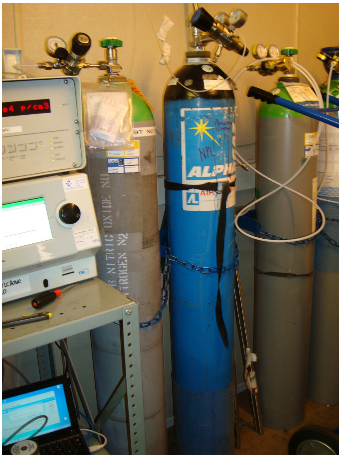
Figure 23: Photograph of nitrogen cylinder supplying gas to the CAMs employing photoionisation detectors, and for the pneumatic control of valves in all four CAMs.
