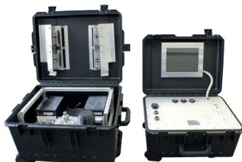
The transportable system offers the possibility of using different columns with pressure ranging from 10 to 400 bars and flow ranging from 0.50 to 10 ml/min. The temperature of the oven can be set up to 100 °C. In addition, different detectors can be added to the system for other applications.
