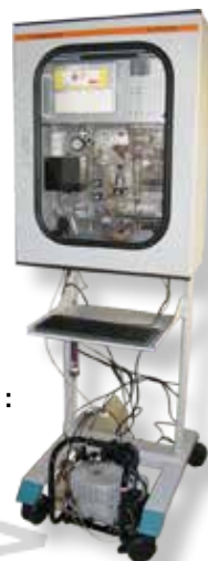
Baie GC Process
