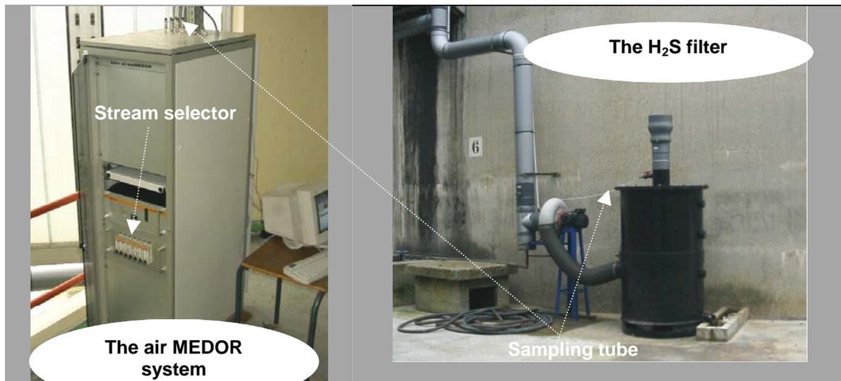
The air MEDOR is a continuous gas chromatograph dedicated to the sulphur compound analysis. The model complies with the norms ISO 6326/2 and DIN 51855/7, for H<sub>2</sub>S/MeSH/DMS/DMDS..... A unique electro-chemical detector allows the specific detection of sulphur species.
