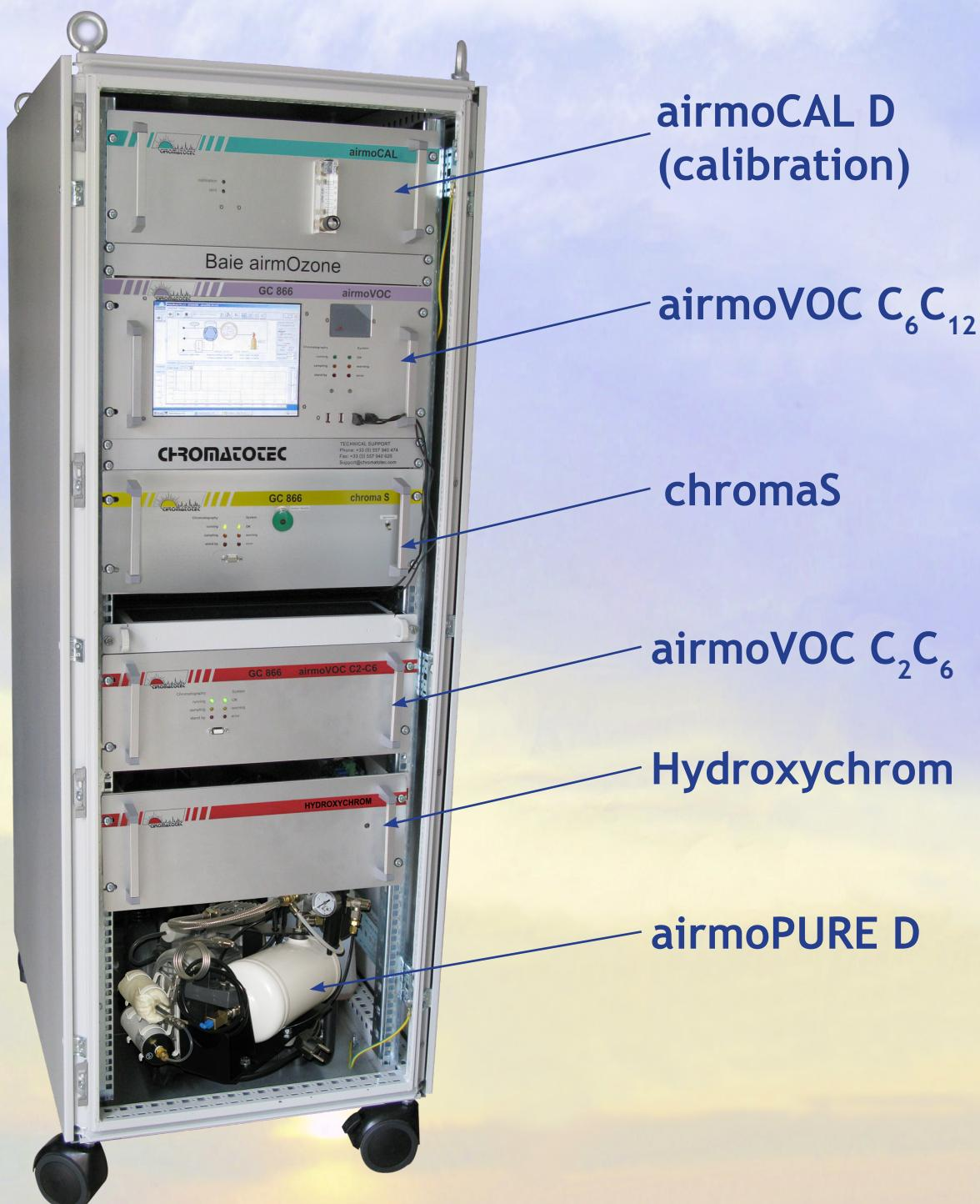
airmOzone  $\text{C}_2\text{C}_{12}$  PAMS 56: complete unit to analyse 56 compounds
