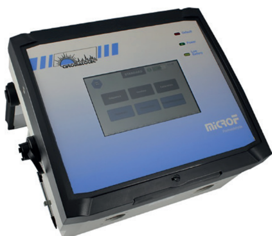
Figure 1: MicroF: Microfluidic formaldehyde analyser
