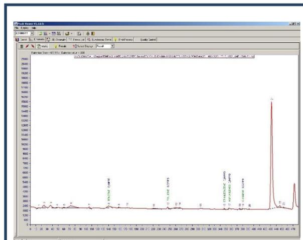
Figure 1 - chromatogram of 476 ml of ambient air (Bordeaux area)
