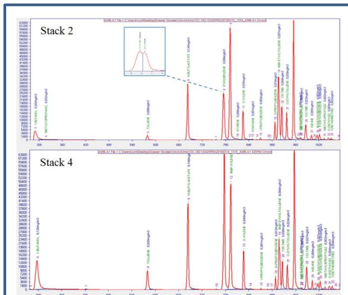
Fig. 1: GC-FID chromatogram (detector value vs retention time) view with PeakViewer software for VOCs emission profiles at stack 2 and stack 4.
