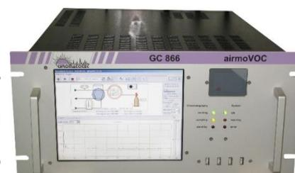
VistaCHROM software allows easy data acquisition and treatment. Reference substance tables included allow the automatic identification of the target compounds by the retention time of the peaks obtained in the chromatograms. Moreover, validation of the results is assured by the internal calibration system and data can be transferred automatically using Modbus or remote control.
