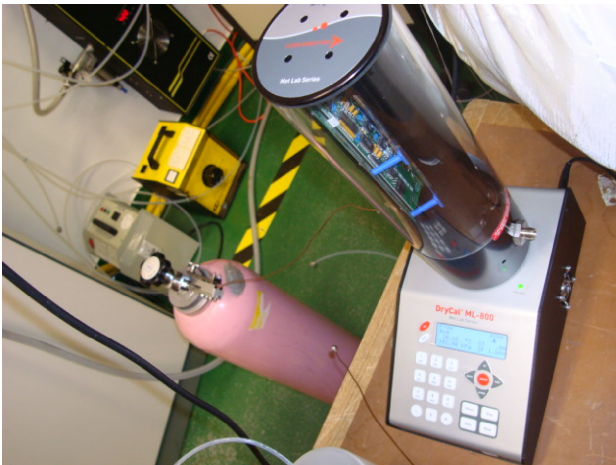
Figure 14: Photograph showing the flow rate calibration system and one of the “Restrictor” valves employed to introduce the determinands from the NPL Standard Gas Mixtures into the sample manifold.
