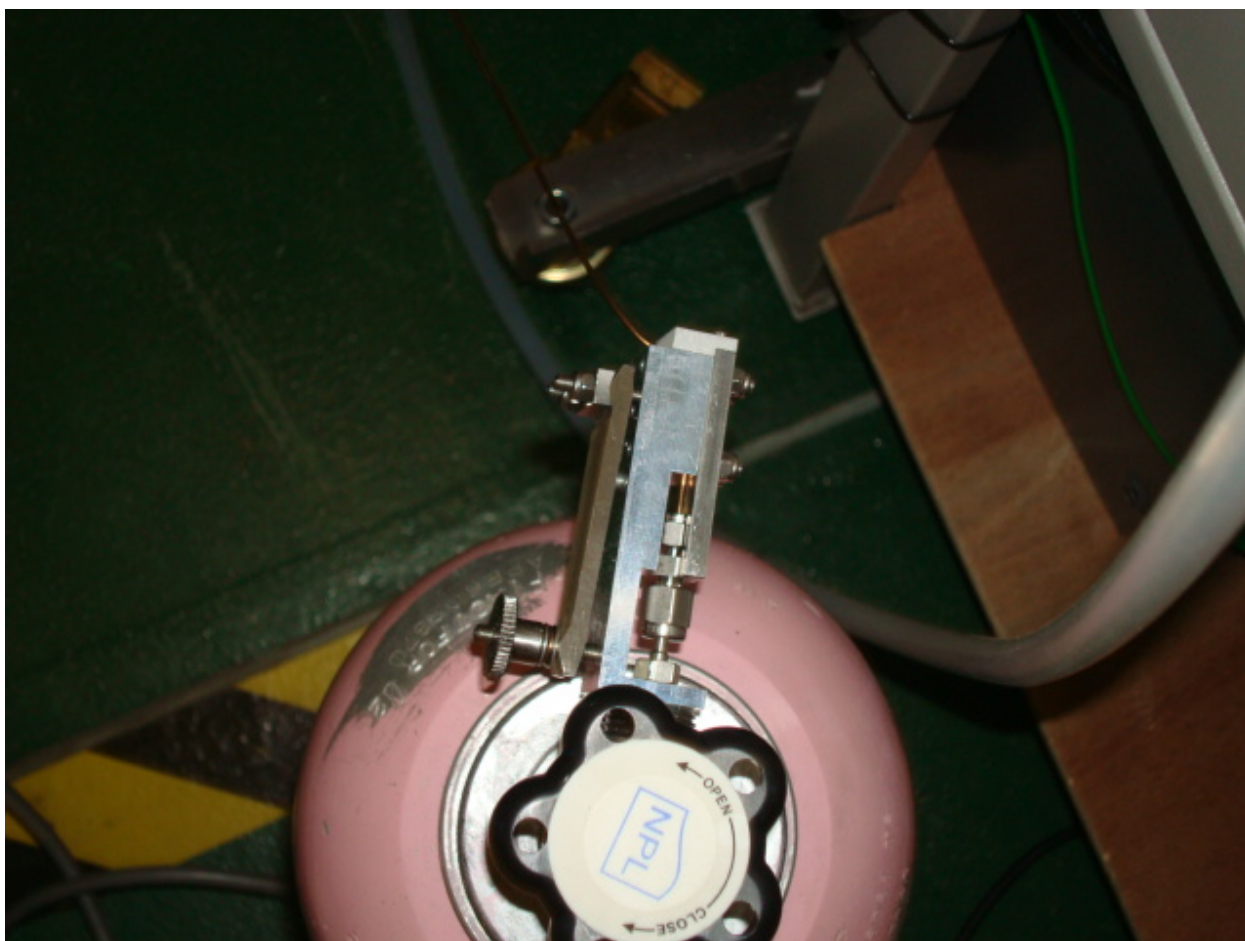
Figure 15: Photograph showing a close-up of a “Restrictor” valve coupled to a Standard Gas Mixture.
