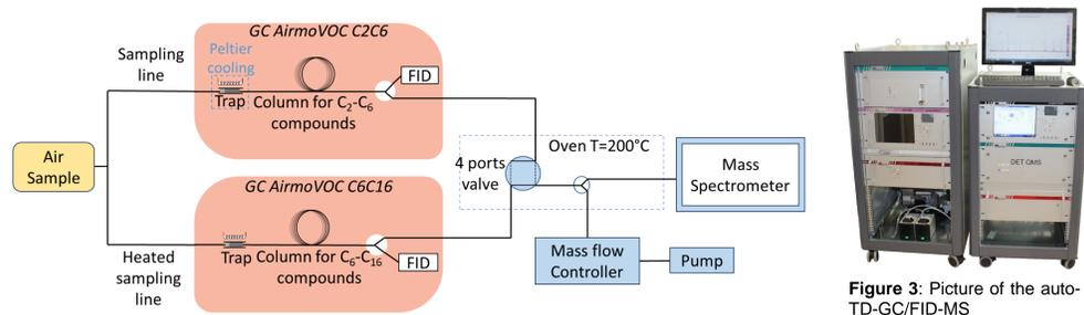
Figure 2: Schematic representation of the auto-TD-GC/FID-MS
