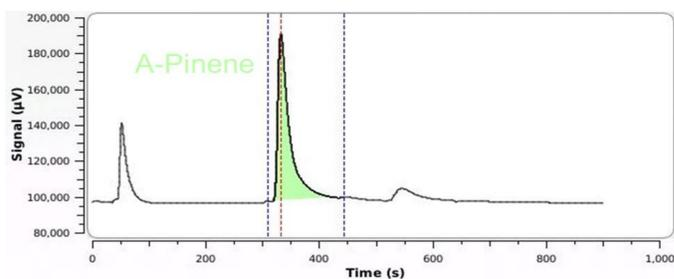
Figure 8: Chromatogram obtained for the analysis of pine tree on the portable analyzer
