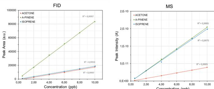
Figure 5: Linearity curves obtained on FID for acetone, alpha-pinene and isoprene
