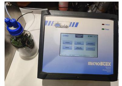
Figure 7: Analysis of pine tree with the micro-GC
