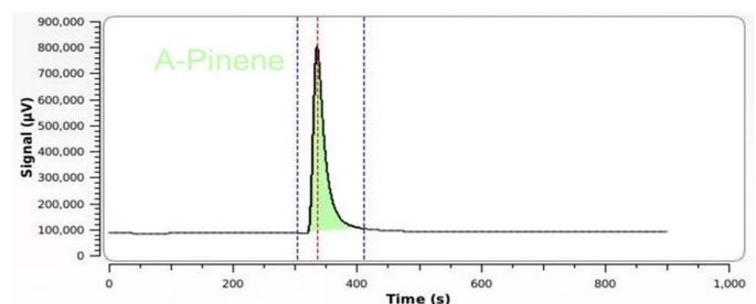
Figure 9: Chromatogram obtained for the analysis of pure alpha pinene
