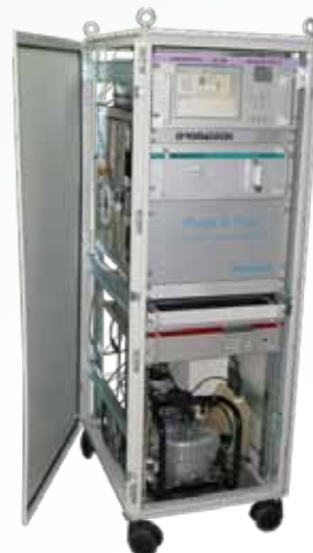
Purge & Trap cabinet
