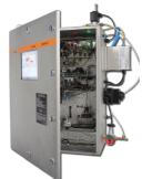
chromaPID or airTOXIC allow online VOCs measurement with our analyzer in Exp version. Thanks to these process-GC analyzers using PID detection we can analyze Benzene alone at ppm level for hygiene or quality control of gases. BTEX and Styrene in ambient air can be monitored in hazardous areas at ppt and ppb levels for air quality monitoring and many VOCs per request.
