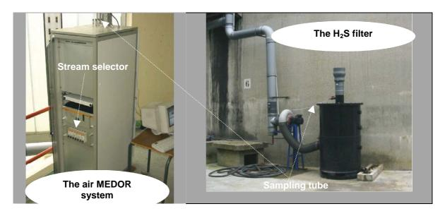
The air MEDOR is a continuous gas chromatograph dedicated to the sulphur compound analysis. The model complies with the norms ISO 6326/2 and DIN 51855/7, for  $H_2S/MeSH/DMS/DMDS....$ . A unique electro-chemical detector allows the specific detection of sulphur species.
