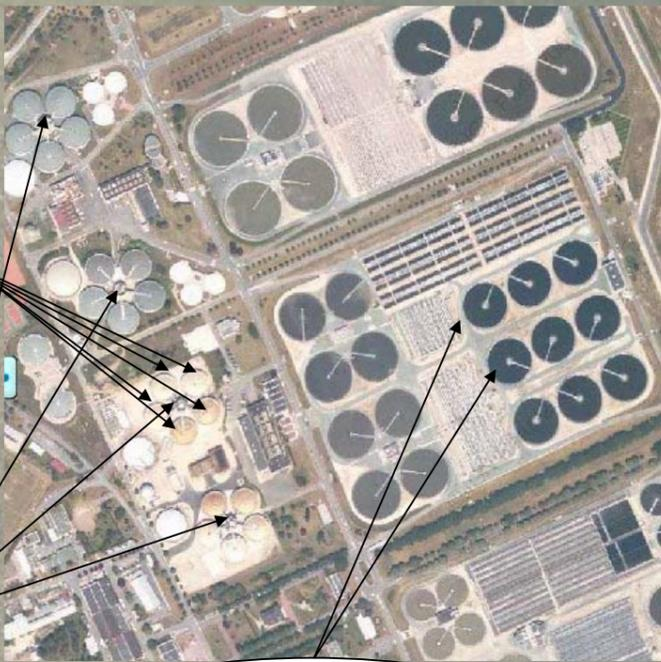
Primary setting tanks placed just before the digestors
